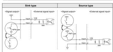
When 24V is applied on Input+ and 0V is applied on Input-, the signal becomes HIGH.
