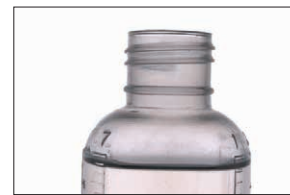
It is possible to form an image of the liquid level without surface reflection.
