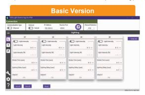
Basic lighting settings such as intensity value and light emission time, as well as trigger input / output settings.
